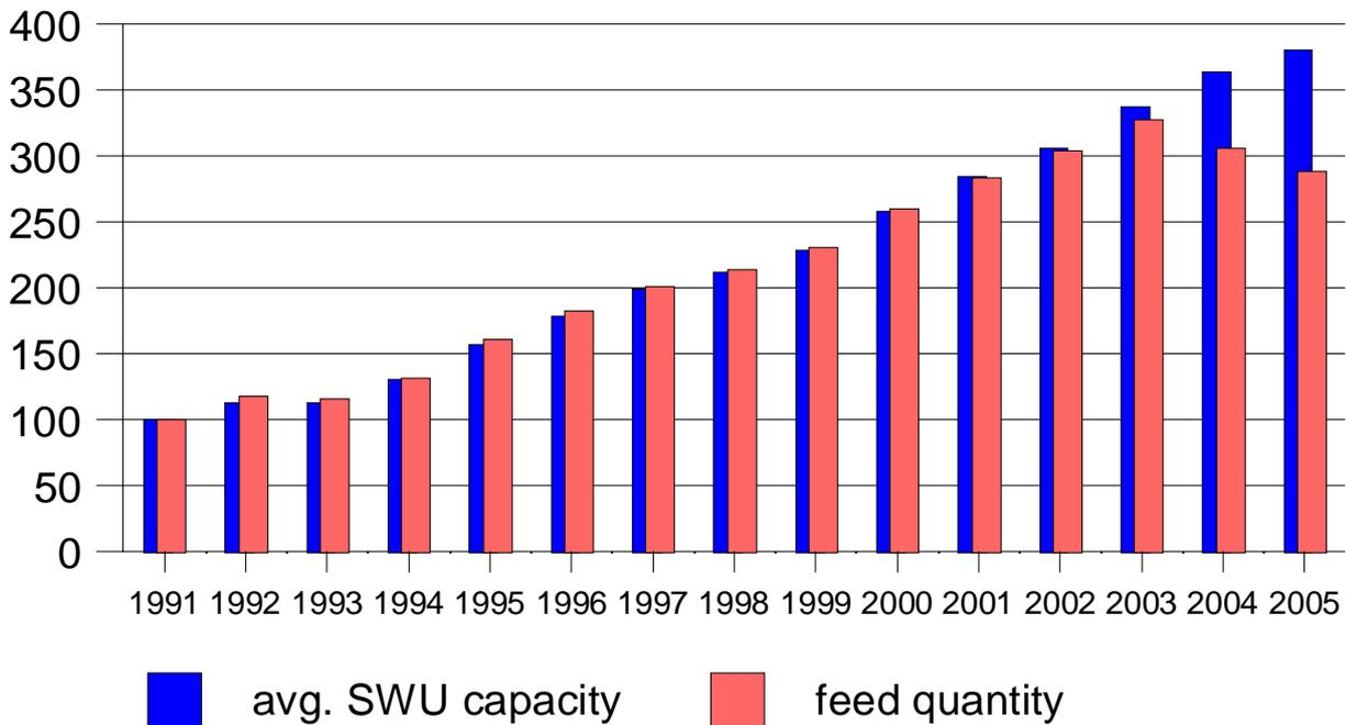
Fig. 1: Urenco Gronau feed-capacity balance (after [Urenco 2006])
